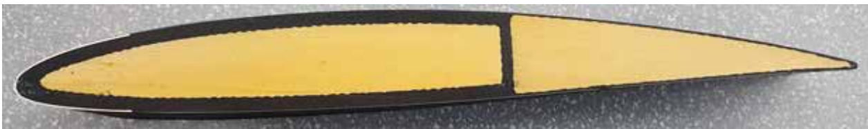
ASC-II Composite Blade Cross-section Figure 2-4
