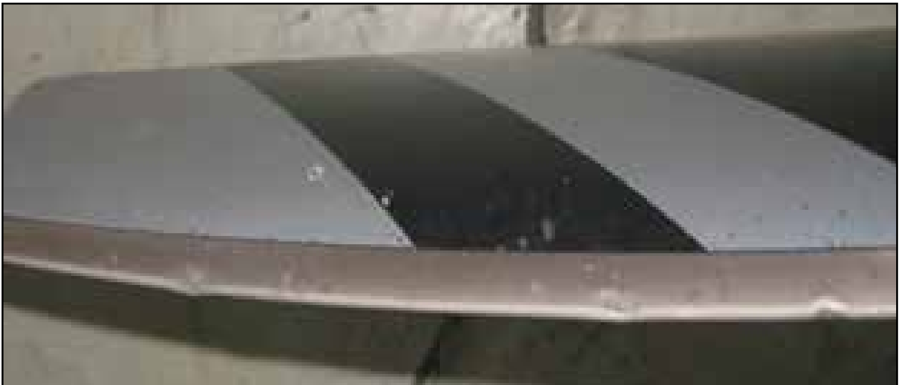
Example of Airworthy Damage to a Composite Blade Figure 2-5
