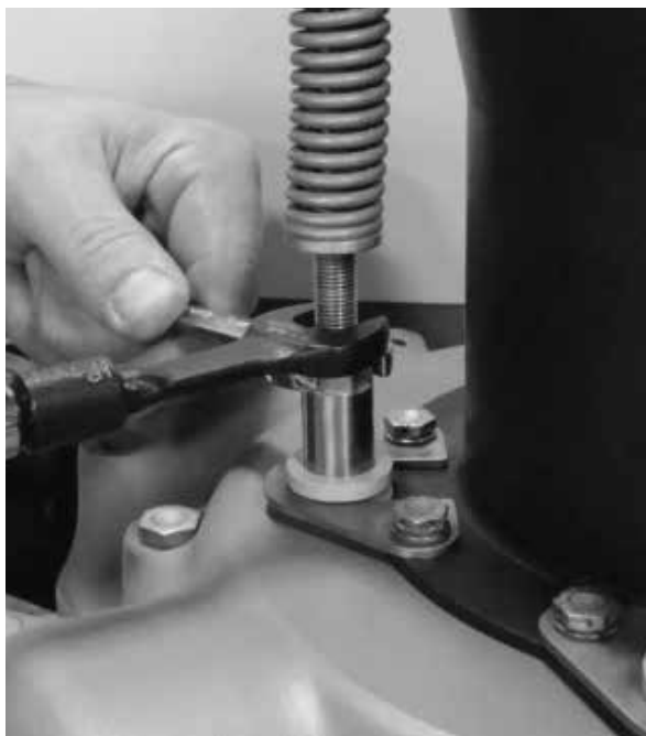
Setting Low Pitch Blade Angle and Beta Ring Run-out Figure 7-55
