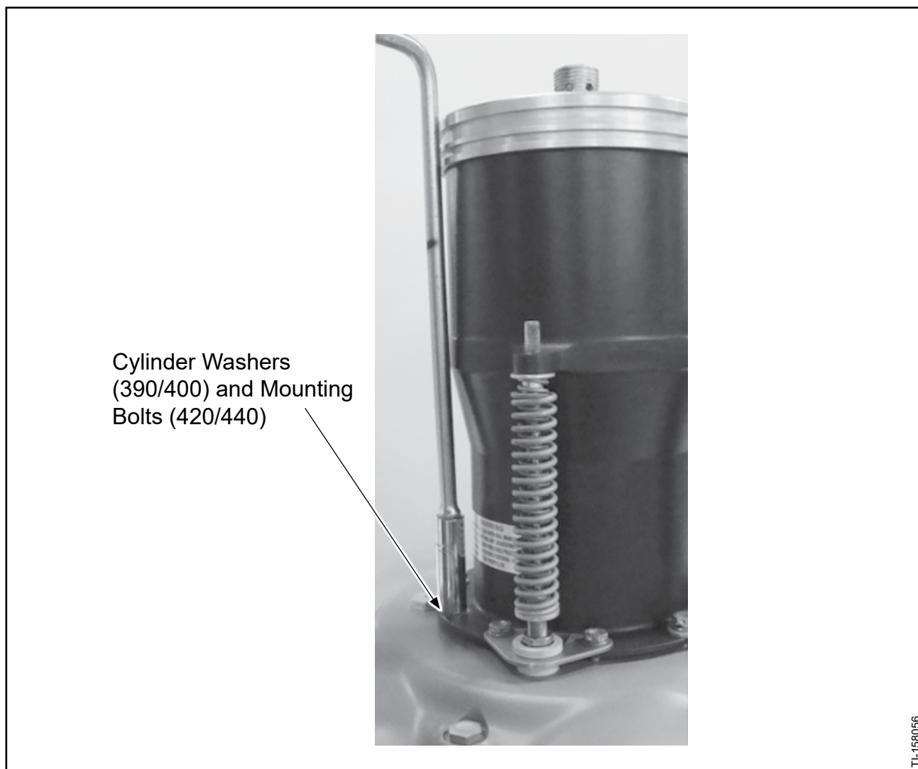
Installing the Cylinder Mounting Bolts Figure 7-43
