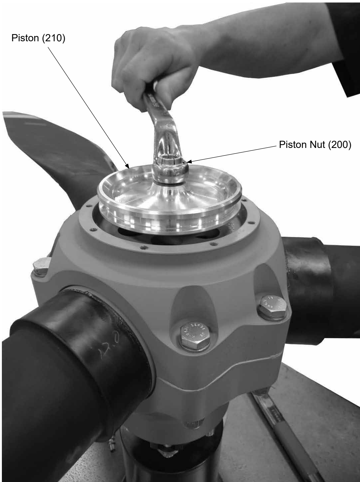
Piston Installation Figure 7-13
