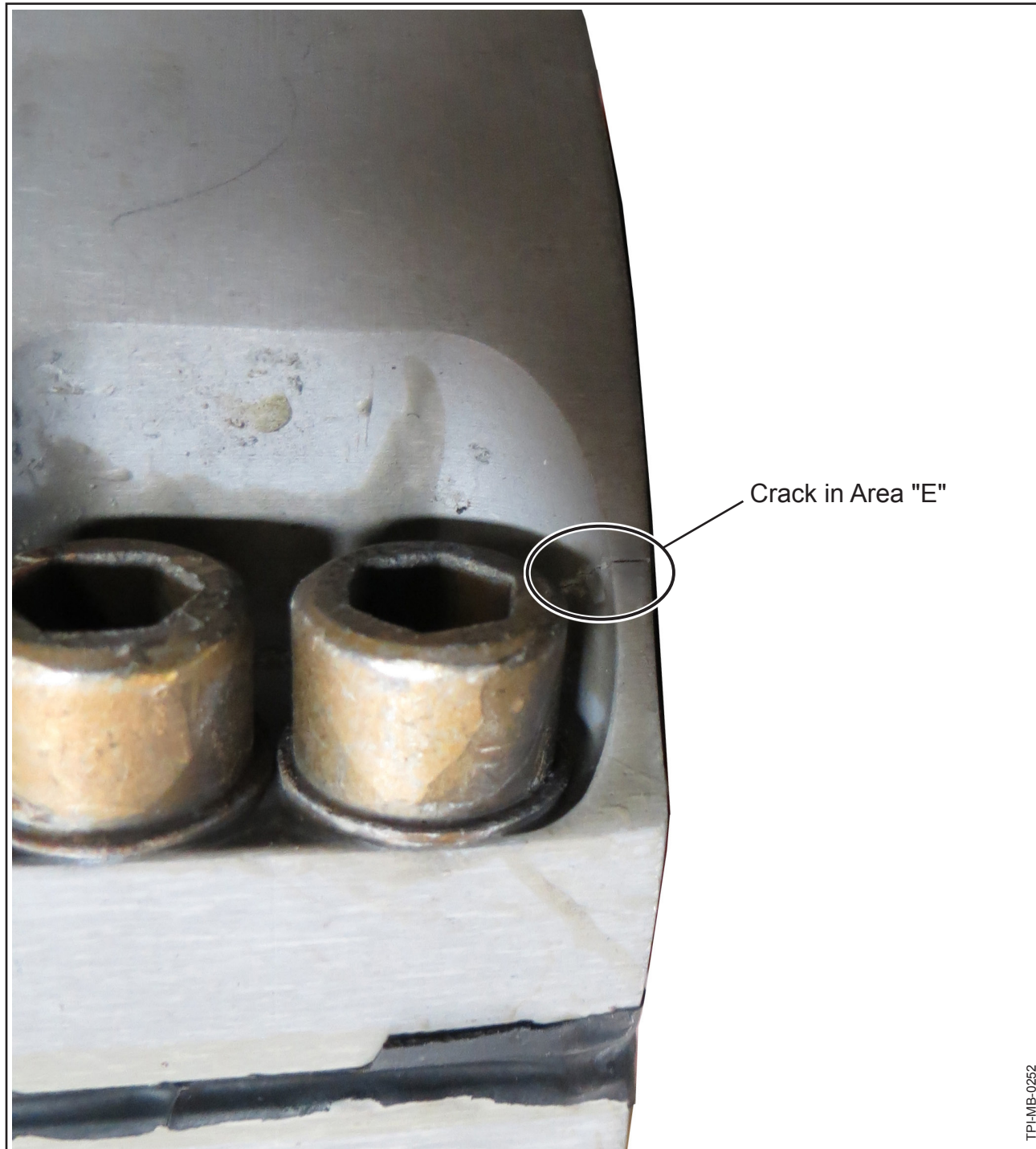
Example of a Cracked Counterweight Clamp Figure 2
