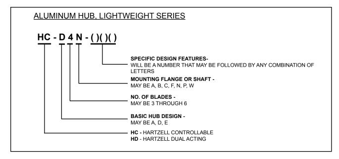
Aluminum Hub Propeller Identification -Lightweight Series Figure 3
