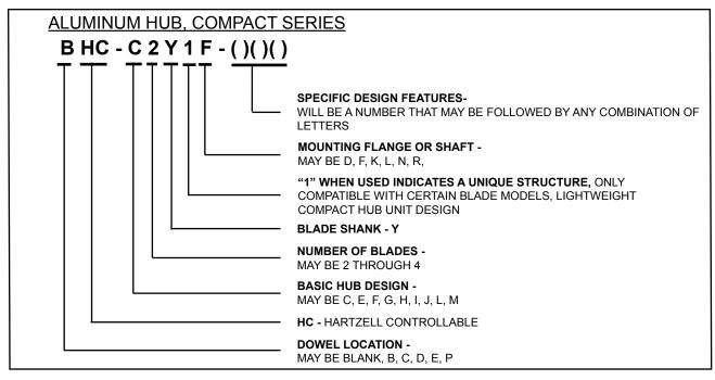
Aluminun Hub Propeller Identification - Compact Series Figure 2
