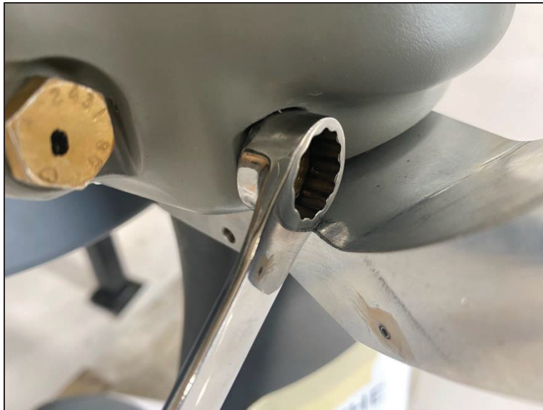
Figure 1 Bolt access under blade counterweight
