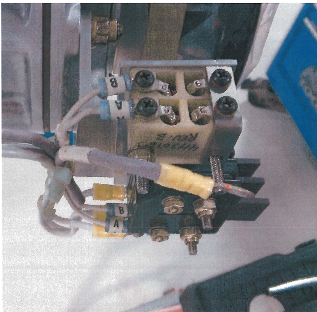
Figure 6 Install MOV and attach MOV wires
