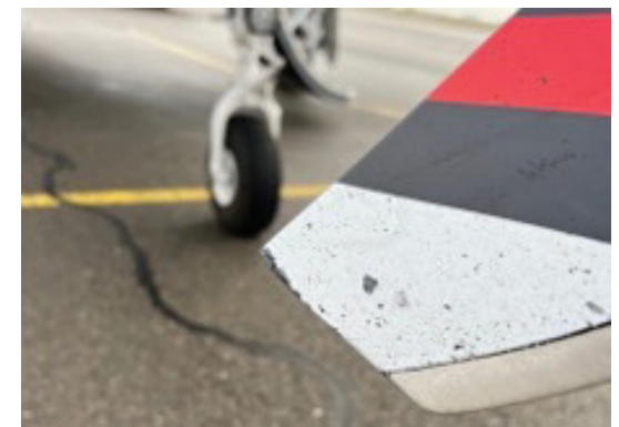
Examples of airworthy damage to composite blades
