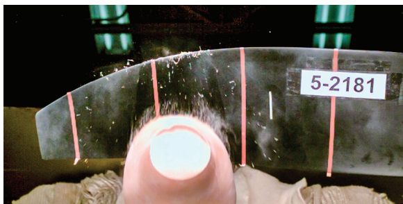
Bird strike testing with 4-lbs weight
