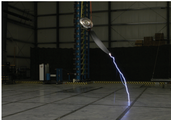
High-voltage lightning strike testing
